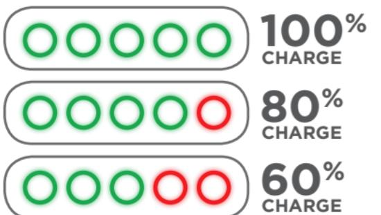
FIGURE 5: EXAMPLE OF FLASHING SEQUENCE INDICATING BATTERY CHARGE LEVEL
