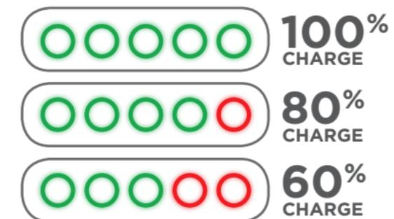
FIGURE 11: EXAMPLE OF FLASHING SEQUENCE INDICATING BATTERY CHARGE LEVEL
