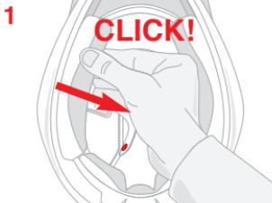
To remove the cheek pads, grip them at the front near the helmet chin strap and pull in the direction of the arrow to free them from the press studs (1).
