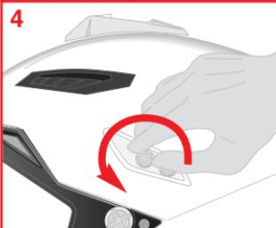
To remove the plastic plates, starting from one side of the helmet, loosen the screws by hand or using a screwdriver (2). Repeat the operation on the other side and then install the canopy.
