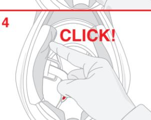
Insert the plastic band between the EPS shell and the outer shell, moving in the direction indicated by the arrow and pressing the press studs in place (4). Check that the cheek pads are perfectly secured to the helmet.
